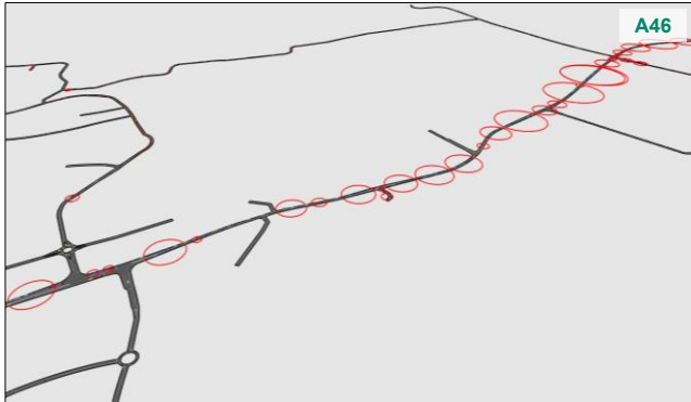
Figure 29: Model Snapshots of the A46 approach to the A46 / Loverose Way / Northway Lane signalised junction, AM Peak Period (08:40 hours)
