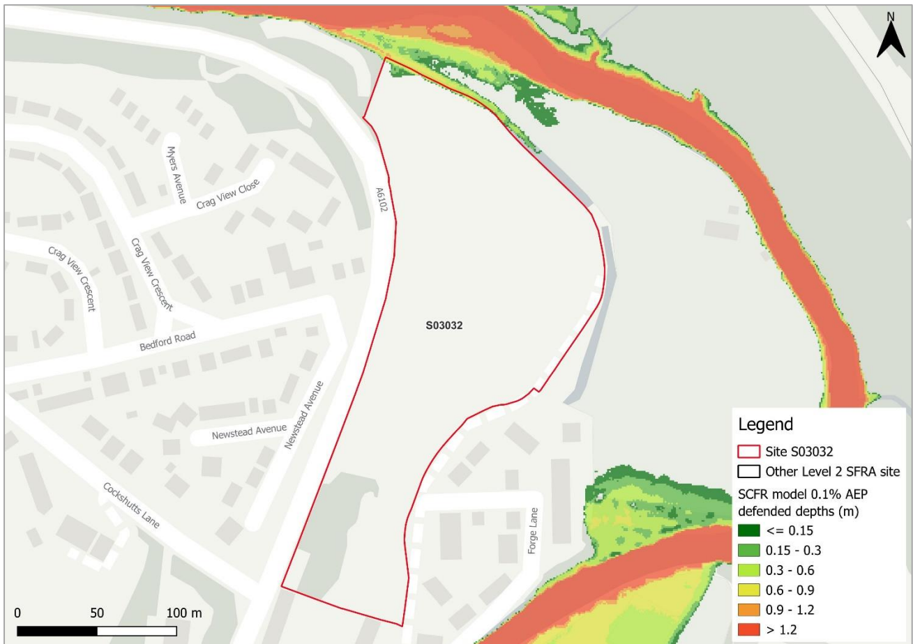
Figure 2-4: Flood depths for the present day 1% AEP defended flood event
