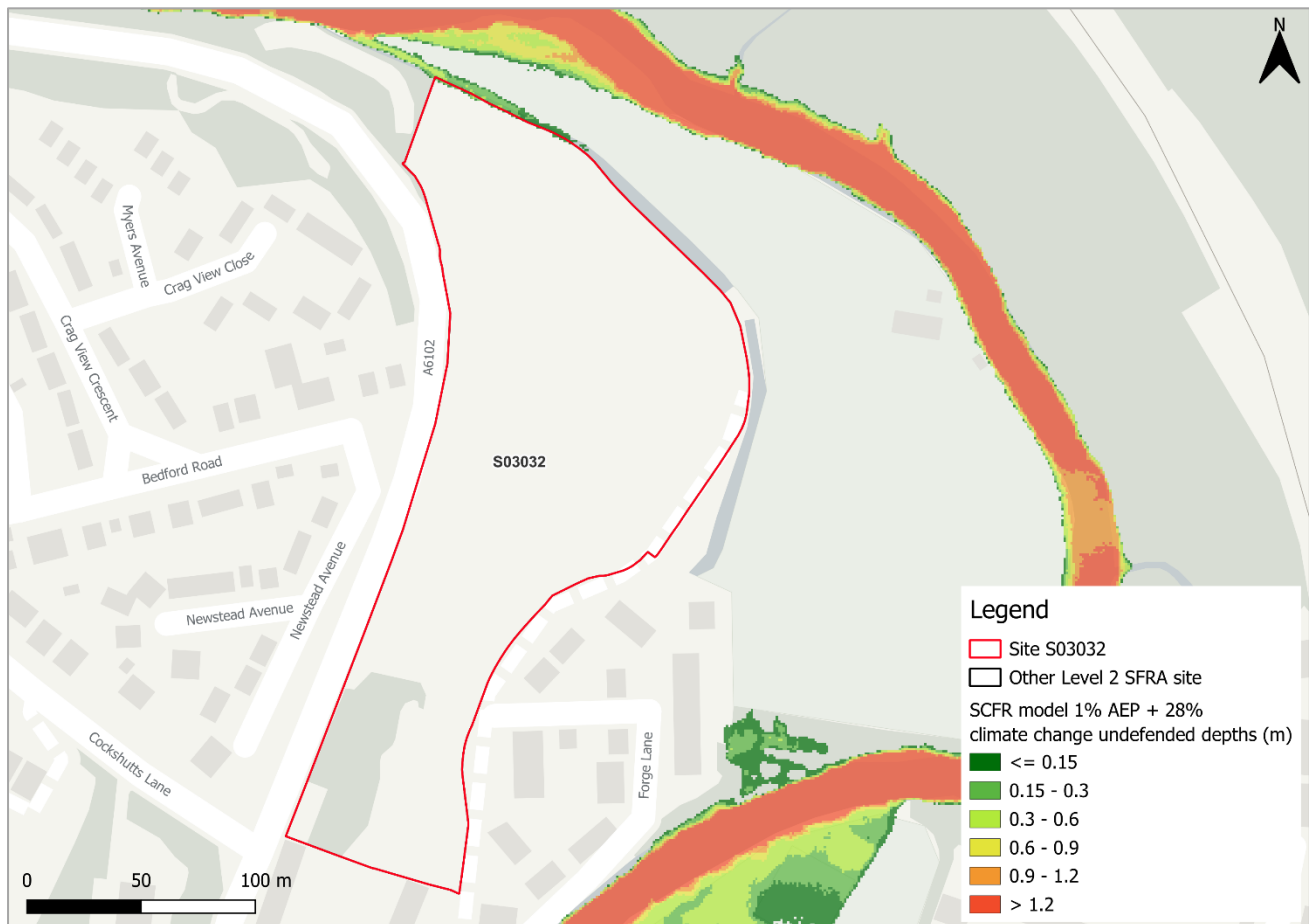
Figure 2-3: Flood depths for 1% AEP undefended flood event +28% (central climate change allowance)
