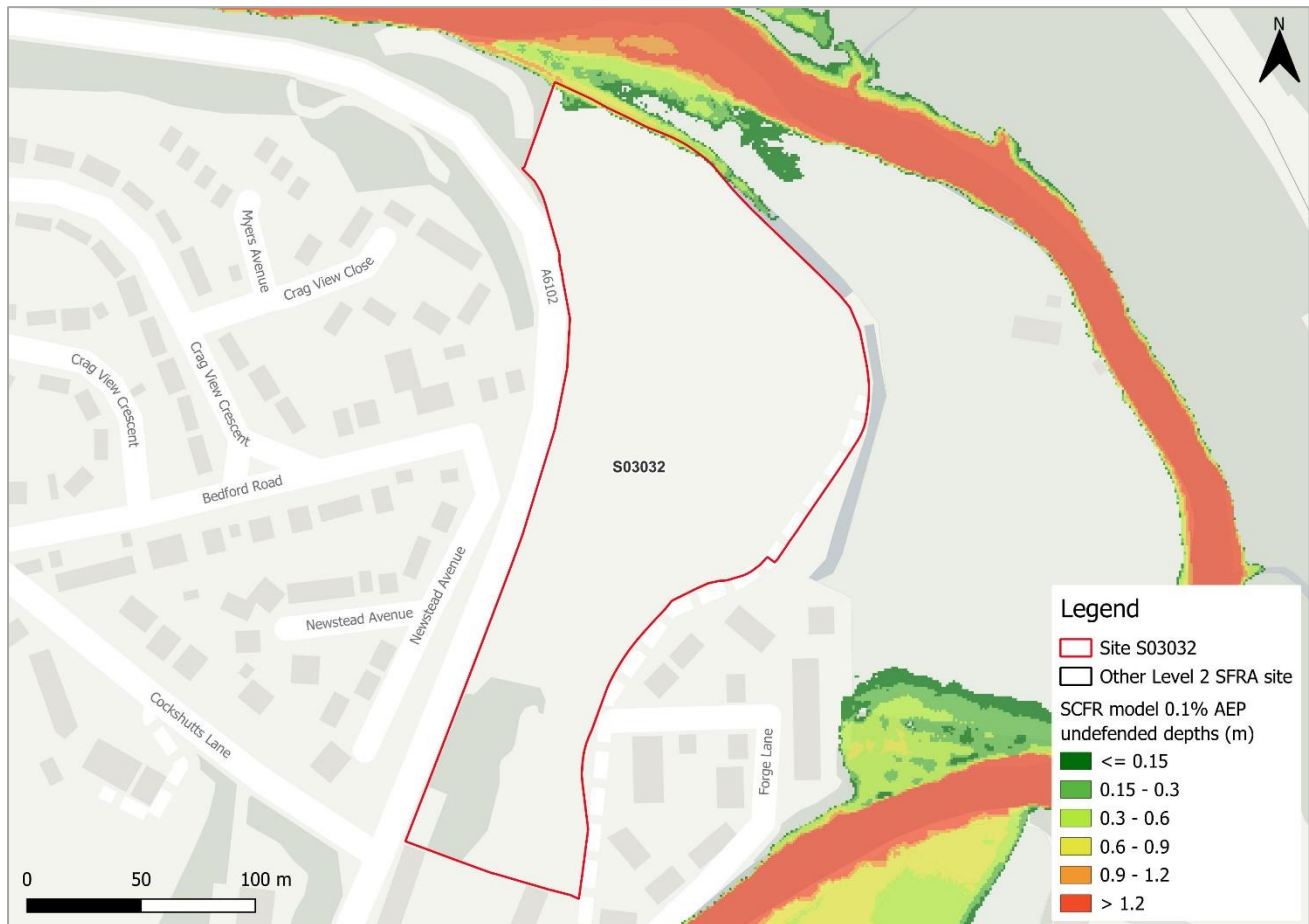
Figure 2-2: Flood depths for 0.1% AEP undefended flood event
